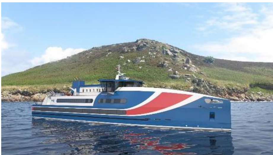
Damen DRPa7213 RoRo modified to take the ground and moor stern to a ramp.
